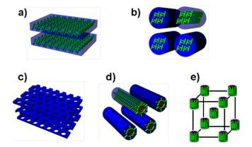
**FIGURE 4** Schematic representation of self-assembly of (a) monolayer structure for **1a**, (b) rectangular columnar structure for **1b**, (c) perforated lamellar structure for **2a**, (d) oblique columnar structures for **2b**, **2c**, **2d**, and (e) the body-centered tetragonal superlattice for **3a**, **3b**. [Color figure can be viewed in the online issue, which is available at wileyonlinelibrary.com.]
