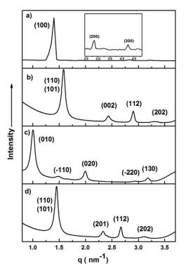
FIGURE 2 Small-angle X-ray diffraction patterns of the rod-coil oligomers measured in their solid state; (a) 1a, (b) 3a, (c) 1b, and (d) 3b.
