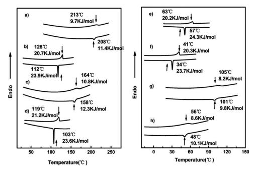
FIGURE 1 DSC traces (10 °C/min) recorded during the second heating scan and the first cooling scan of the series of Compounds 1, 2, and 3; (a) 1a, (b) 2a, (c) 1b, (d) 2b, (e) 2c, (f) 2d, (g) 3a, and (h) 3b.
